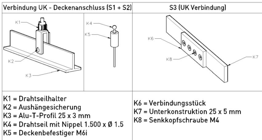
**Beispielschema designed acoustic baffle fibercomfort**
