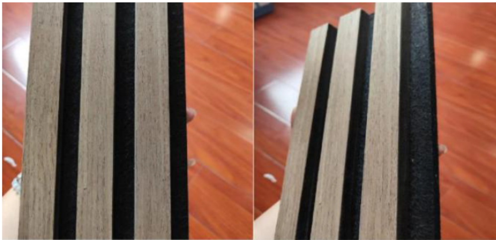
Figure 1: Wooden slats acoustic panel G1 from Suzhou Deco Sound New Materials Technology Co., Ltd.
